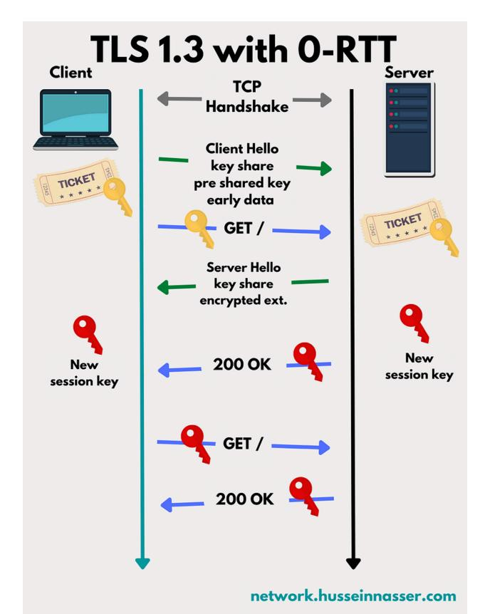
This allows for the application to immediately send its request before the TLS session is even established, yes we still need to establish the TCP connection in case of HTTP/2 or HTTP/1.1 but with HTTP/3 it is a true 0-RTT as QUIC connection establishment and TLS is done in same round trip.
